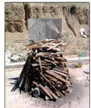
**Figure 2: Test body covered with wood**
