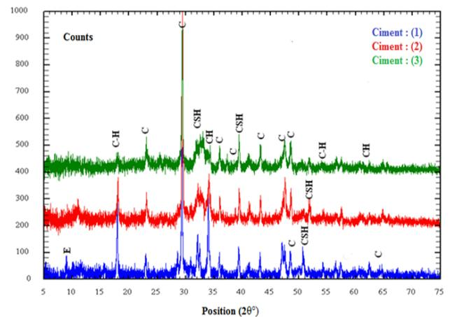
Figure 8: X-ray diffraction of cement pastes 1, 2 and 3
