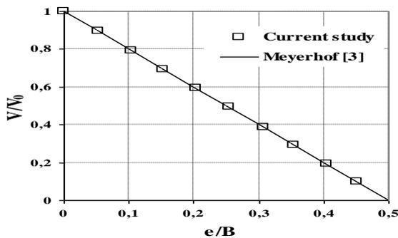
Figure7: Normalised limit load  $V/V_0$  versus  $e/B$  ratio.
