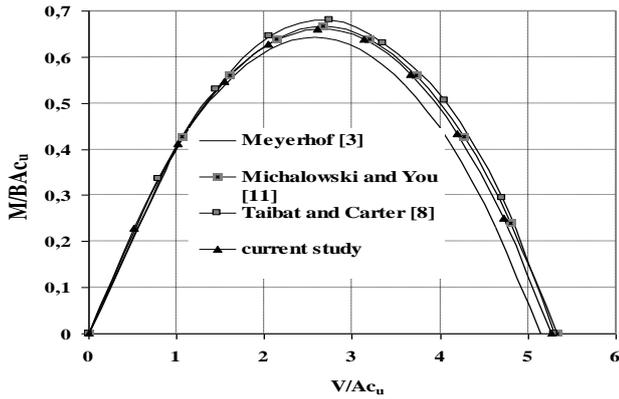
Figure 5: Non-dimensional failure envelopes in  $(V, M)$  plane.
