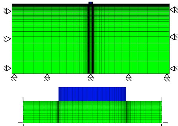
Figure3: Mesh of the numerical model ; (a) : the entire model with the boundary conditions, (b) : mesh in vicinity of the foundation.
