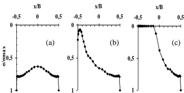
Figure6: Normalized normal stress distribution at the soil-foundation interface ; (a) : non-eccentric loading, (b) :  $e/B = 0.1$ , (c) :  $e/B = 0.25$ .
