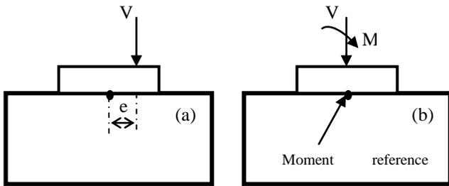
Figure1: Eccentric loading of a surface footing; (a): eccentric loading, (b): equivalent V-M loading.
