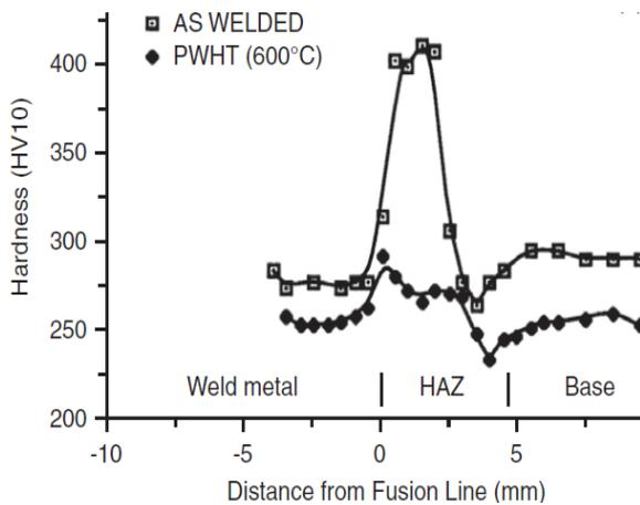
Figure 3: Profile of Vickers hardness before PWHT and after PWHT of 2 hours at 600°C
