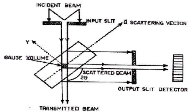
Figure 4: Neutron Diffraction Experimental Setup
