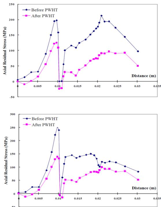
**Figure7: Axial residual stress in weld area at 157.5 and 337.5 degree from welding start point**
