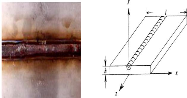
Figure1: Schematic diagram of the welding test plate
