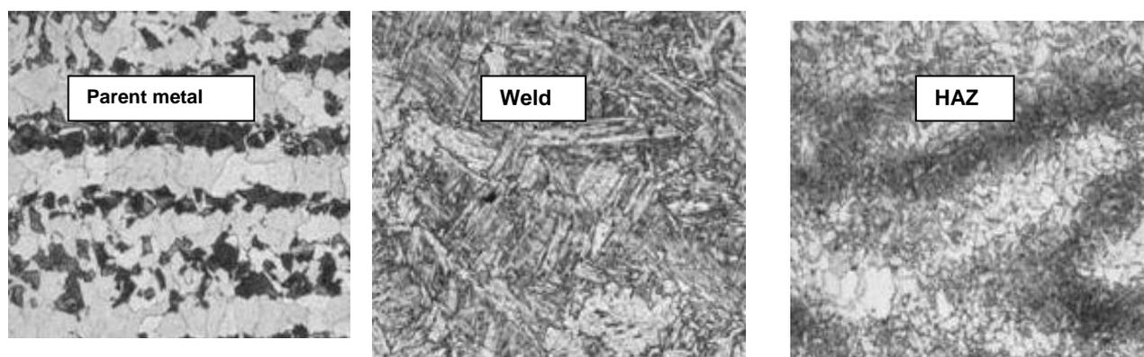
Figure2: Optical micrographs through welded section after PWHT
