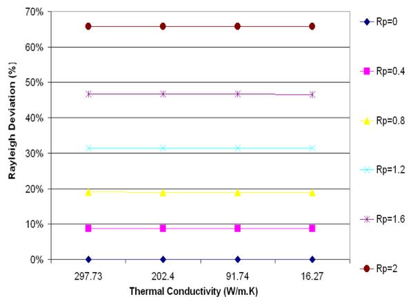
**Figure 15 :** Channel Rayleigh number deviation versus the thermal conductivity and aspect ratios of the protuberances for the uniform heat flux of 100 [W/m<sup>2</sup>]
