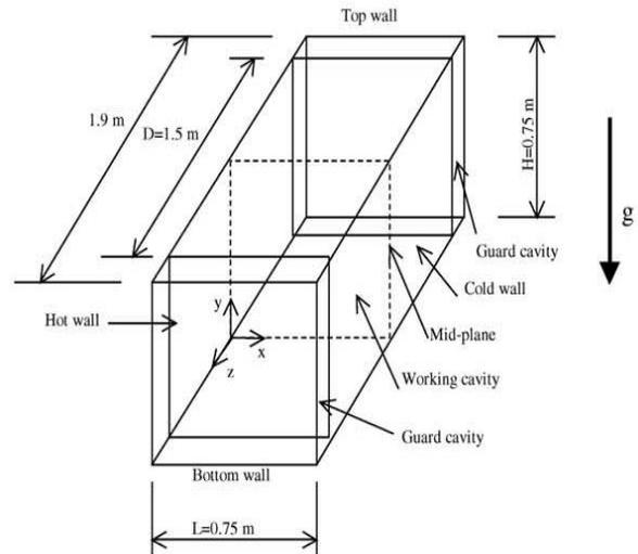
Figure 9 : Experimental three-dimensional schematic diagram of the air filled cavity
