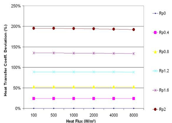
**Figure 16 :** Channel Air heat transfer coefficient deviation versus the applied heat fluxes and aspect ratios of the protuberances for carbon steel protuberances
