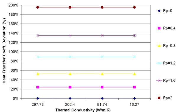
**Figure 13 :** Channel Air heat transfer coefficient deviation versus the thermal conductivity and aspect ratios of the protuberances for the uniform heat flux of 100 [W/m<sup>2</sup>]
