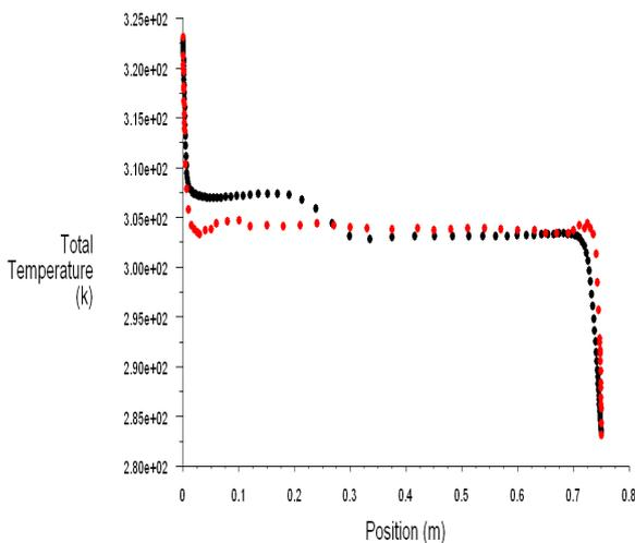
Figure 8: Temperature profile in the middle height of the cavity: comparison computations and experimental data
