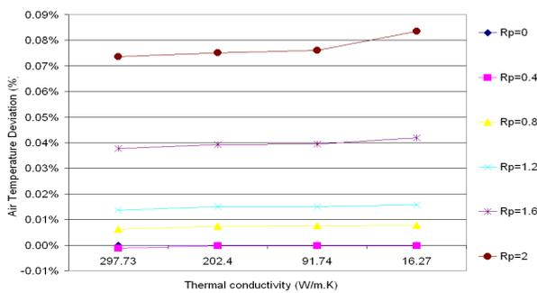
**Figure 12 :** Channel Air temperature deviation versus the thermal conductivity and aspect ratios of the protuberances for the uniform heat flux of 100 [W/m<sup>2</sup>]
