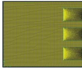
Figure 5: Mesh for 1.2 aspect ratio
