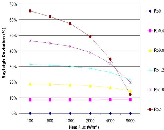
Figure 19: Channel Rayleigh number deviation versus the applied heat fluxes and aspect ratios of the protuberances for carbon steel protuberances
