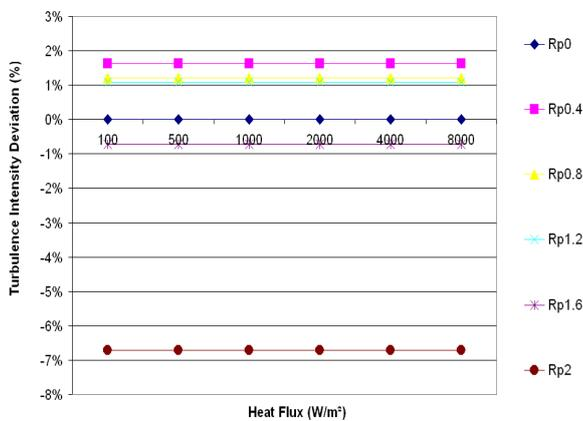
Figure 18: Channel turbulence intensity deviation versus the applied heat fluxes and aspect ratios of the protuberances for carbon steel protuberances
