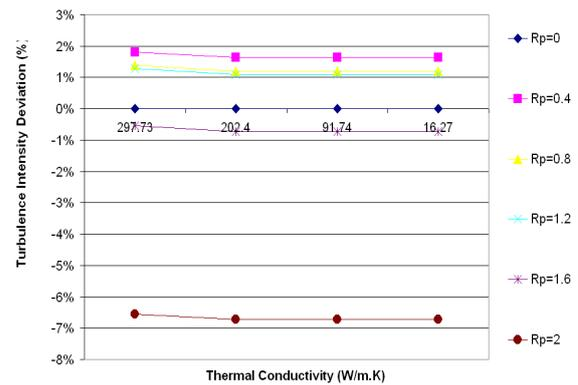
**Figure 14 :** Channel turbulence intensity deviation versus the thermal conductivity and aspect ratios of the protuberances for the uniform heat flux of 100 [W/m<sup>2</sup>]
