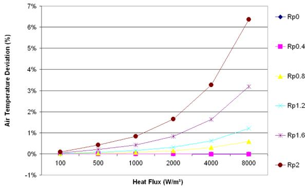
Figure 17 : Channel Air temperature deviation versus the applied heat fluxes and aspect ratios of the protuberances for carbon steel protuberances
