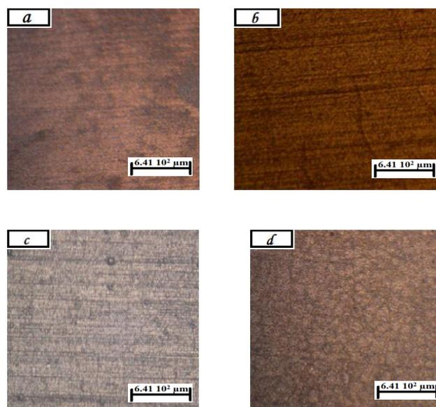
**Figure 01: Optic microscopy images of various coatings electrodeposited at a) 1 A/dm<sup>2</sup>, b) 3 A/dm<sup>2</sup>, c) 5 A/dm<sup>2</sup> and d) 8 A/dm<sup>2</sup>**
