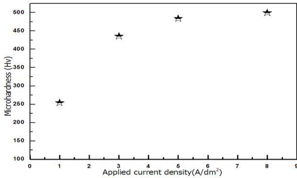
**Figure 03: Variation of microhardness as a function of applied current density**
