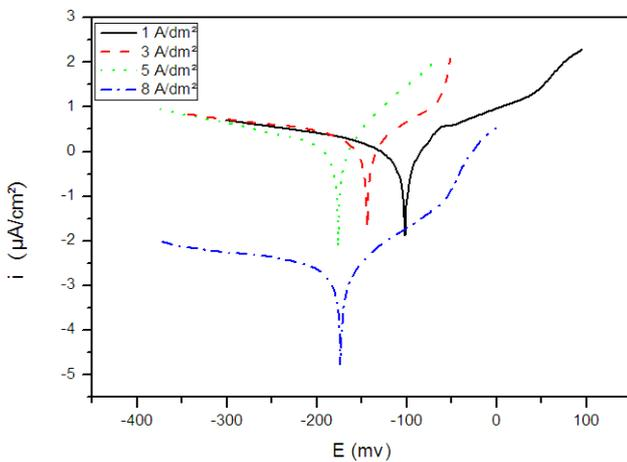
**Figure 04: Polarization curves of Ni-Cr alloy coatings fabricated at different current densities in 0.6M NaCl**
