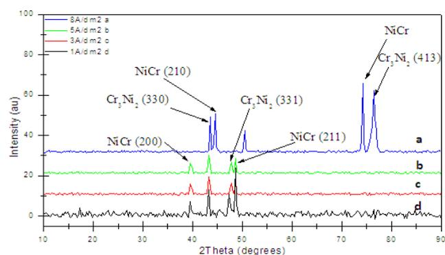
**Figure 02: XRD patterns of Ni-Cr samples as a function of applied current densities**
