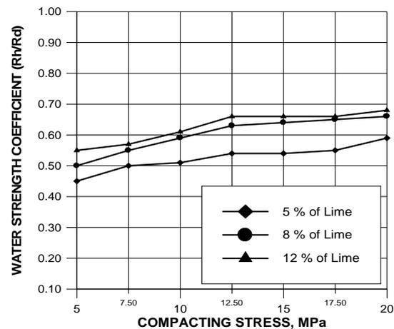
Figure 5 : Influence of compacting force and cement content on the mechanical strength
