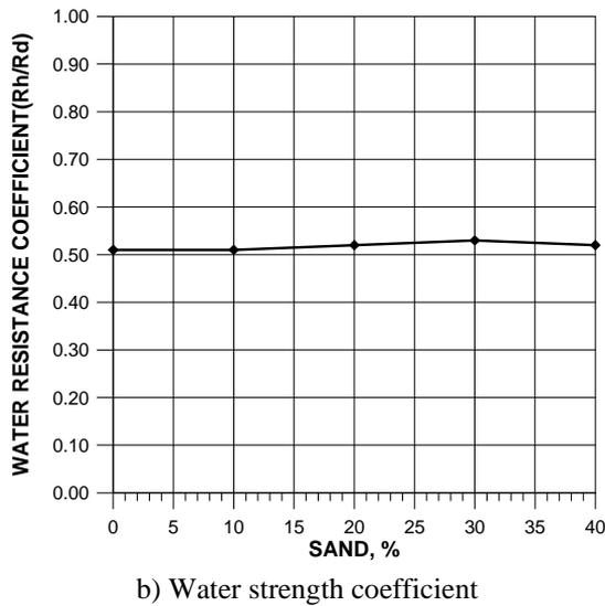
Figure 2 : Sand content influences on compressive strength and water strength. Coefficient with 8% lime stabilizer and 10 MPa compacting stress.
