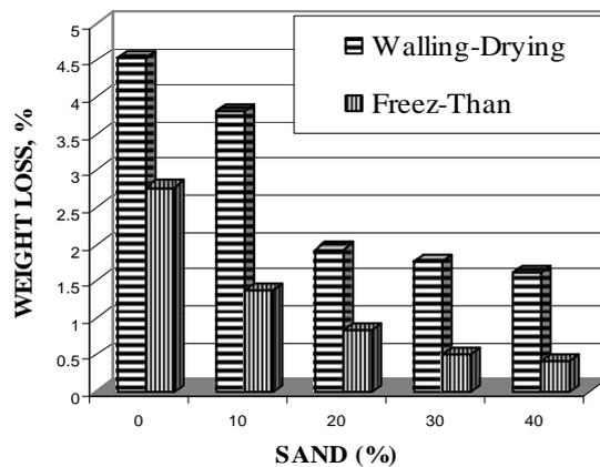
Figure 3 : Influence of sand content on the absorption and loss of weight (8% lime and compacting stress of 10 MPa)
