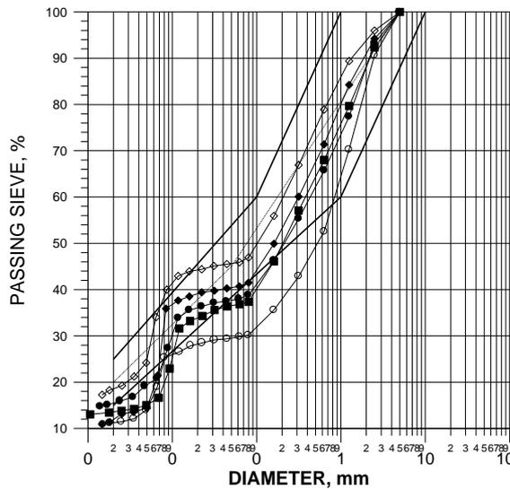
**Figure 1 : Grading curves Aggregate analysis of used soil, corrected soil and the recommended limit zone of stabilized earth concrete.**
