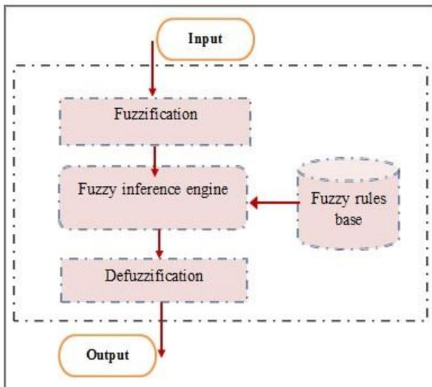
Figure 04: Fuzzy engine architecture
