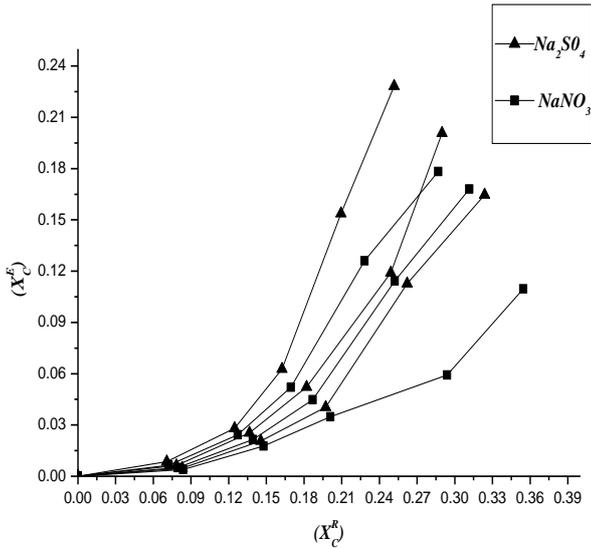
Figure 02c: Comparison of the salting out effect for the system water (a)- cyclohexane (b)- ethanol (c) (Salt-free basis)
