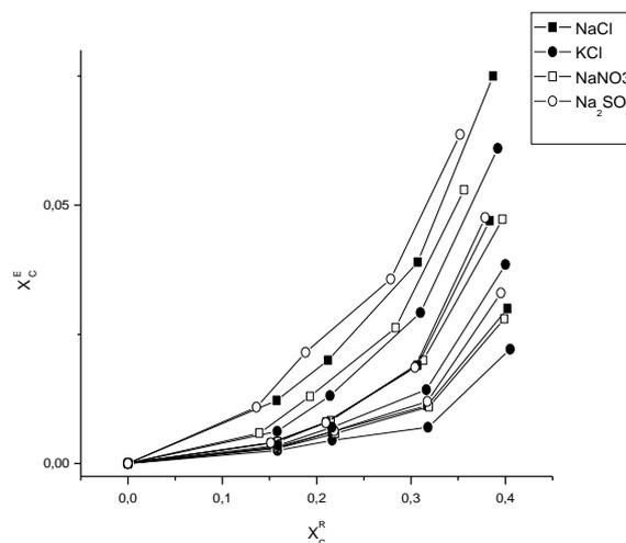
**Figure 01c:** Comparison of the salting out effect for the system water (a) - toluene (b) - acetone (c) (Salt-free basis)
