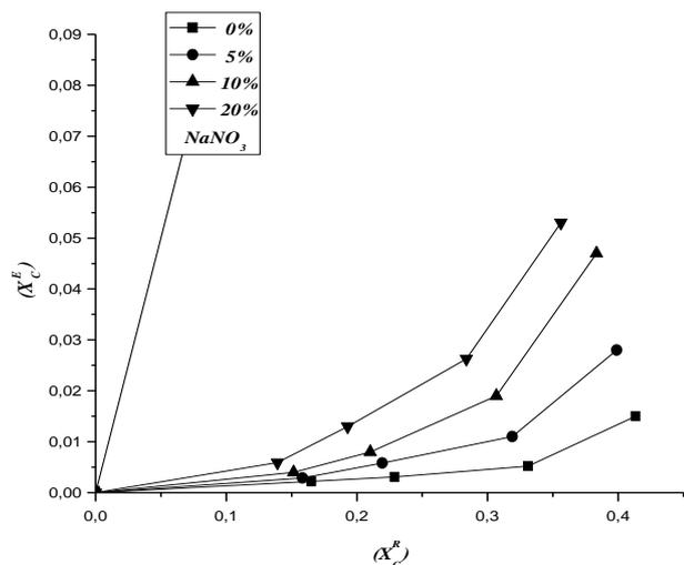
**Figure 4a:** Effect of  $\text{NaNO}_3$  on the equilibrium distributions for different weight percentages for the system water (a) - xylene (b) - methanol (c) (Salt-free basis)
