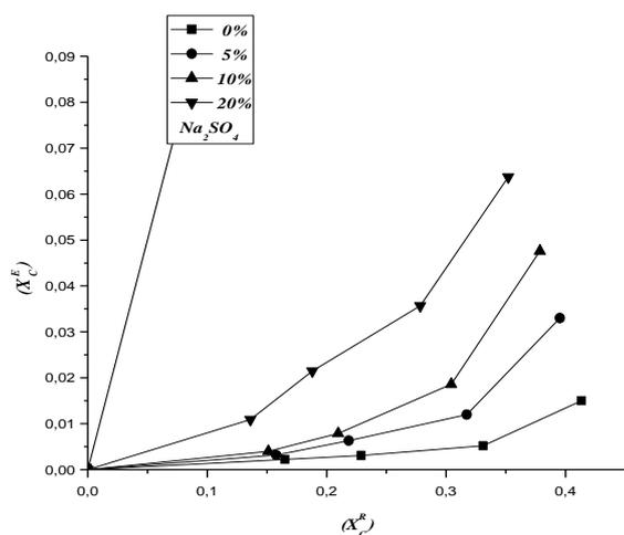
**Figure 4b:** Effect of  $\text{Na}_2\text{SO}_4$  on the equilibrium distributions for different weight percentages for the system water (a) - xylene (b) - methanol (c) (Salt-free basis)
