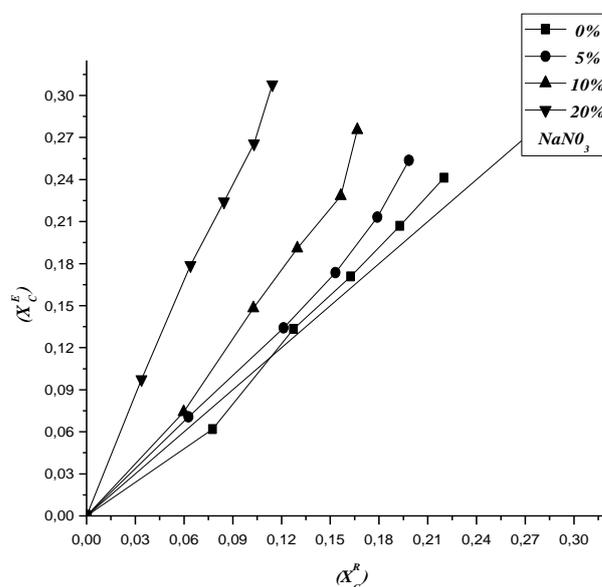
Figure 01: Effect of  $\text{NaNO}_3$  on the equilibrium distributions for different weight percentages for the system water (a)-toluene (b)-acetone(c) (Salt-free basis)
