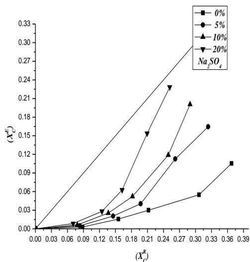
Figure 02b: Effect of  $\text{Na}_2\text{SO}_4$  on the equilibrium distributions for different weight percentages for the system water (a)-cyclohexane (b)- ethanol (c) (Salt-free basis)
