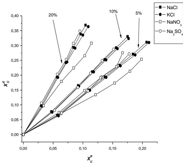
Figure 04c: Comparison of the salting out effect for the system water (a) - xylene (b) - methanol (c) (Salt-free basis)
