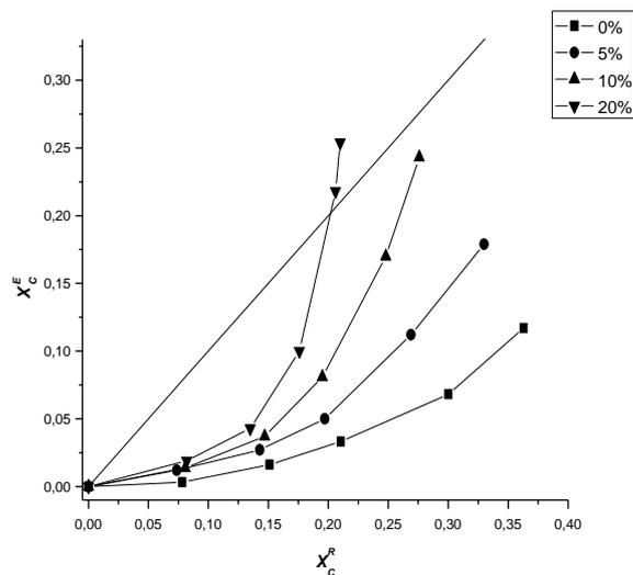
Figure 03a: Effect of  $\text{Na}_2\text{SO}_4$  on the equilibrium distributions for different weight percentages for the system water (a)-cyclohexane (b)- 2-propanol (c) (Salt-free basis)
