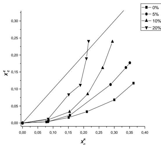
Figure 03b: Effect of  $\text{NaNO}_3$  on the equilibrium distributions for different weight percentages for the system water (a)-cyclohexane (b)- 2-propanol (c) (Salt-free basis)
