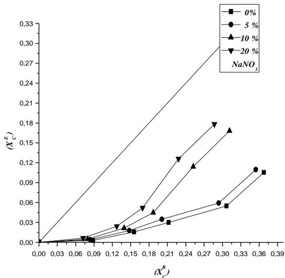
Figure 02a: Effect of  $\text{NaNO}_3$  on the equilibrium distributions for different weight percentages for the system water (a)-cyclohexane (b)-ethanol(c) (Salt-free basis)
