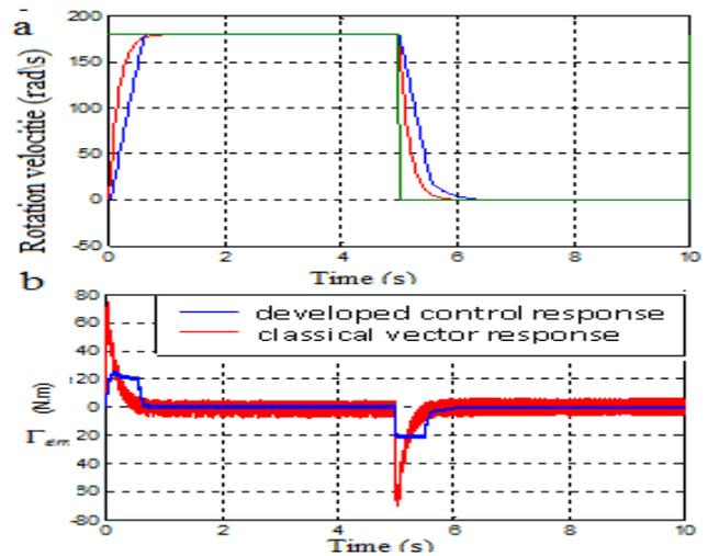
Figure 6: (a) reference and motor angular speed (b) electromagnetic torque
