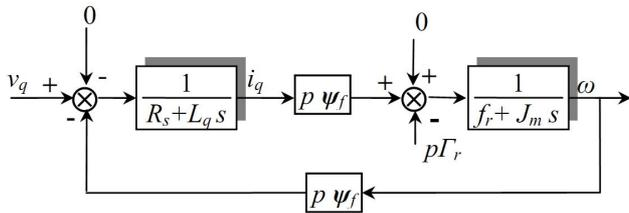
Figure 3: Uncoupled model of studied machine
