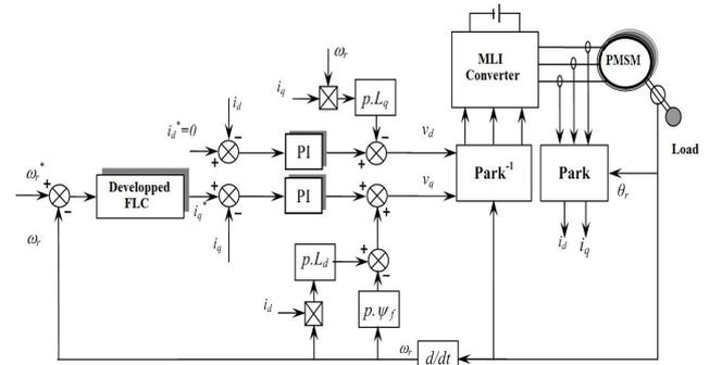
Figure 5: global structure of PM machine Control
