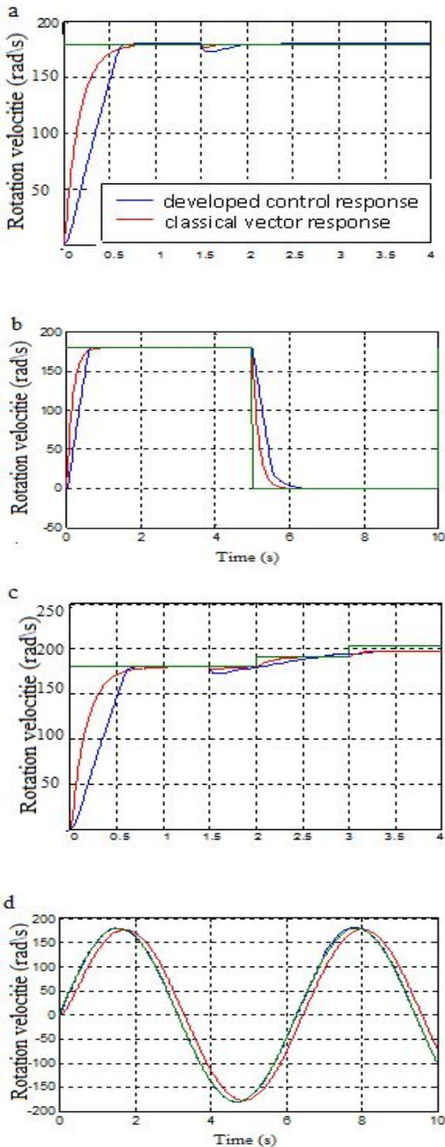
Figure 11: Angular speed of machine with load for difference reference speed
