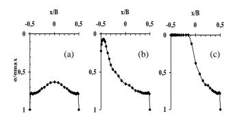
Figure6: Normalized normal stress distribution at the soilfoundation interface ; (a) : non-eccentric loading, (b) : e/B = 0.1, (c) : e/B = 0.25.
