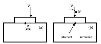
Figure1: Eccentric loading of a surface footing; (a): eccentric loading, (b): equivalent V-M loading.
