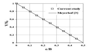
Figure7: Normalised limit load V/V<sub>0</sub> versus e/B ratio.
