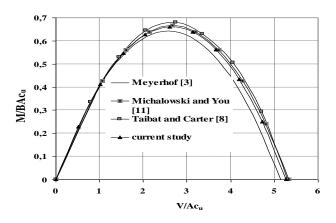
Figure 5: Non-dimensional failure envelopes in (V, M) plane.
