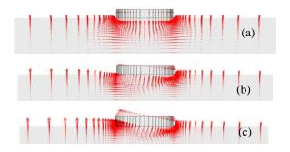
Figure8: Displacement vectors ; (a) non-eccentric loading, (b) : e/B = 0.1, (c) : e/B = 0.25.
