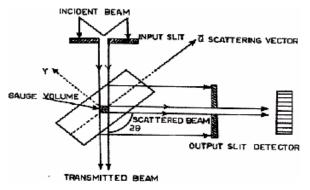
Figure 4: Neutron Diffraction Experimental Setup
