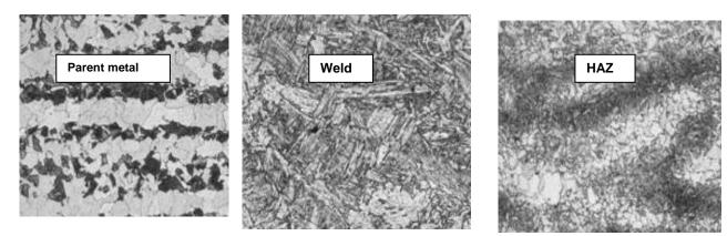
Figure2: Optical micrographs through welded section after PWHT
