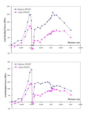
Figure7: Axial residual stress in weld area at 157.5 and 337.5 degree from welding start point
