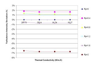
Figure 14: Channel turbulence intensity deviation versus the thermal conductivity and aspect ratios of the protuberances for the uniform heat flux of 100 [W/m2]
