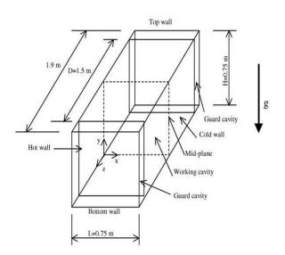
Figure 9 : Experimental three-dimensional schematic diagram of the air filled cavity
