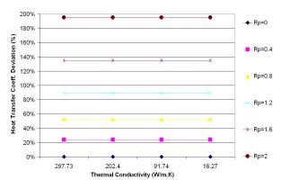
Figure 13 : Channel Air heat transfer coefficient deviation versus the thermal conductivity and aspect ratios of the protuberances for the uniform heat flux of 100 [W/m2]
