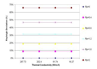
Figure 15: Channel Rayleigh number deviation versus the thermal conductivity and aspect ratios of the protuberances for the uniform heat flux of 100 [W/m2]
