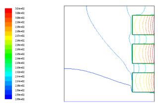
Figure 11 : Air temperature inside the Vertical channel for the case 20
