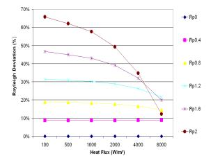
Figure 19: Channel Rayleigh number deviation versus the applied heat fluxes and aspect ratios of the protuberances for carbon steel protuberances
