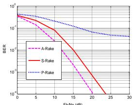
Figure 07: BER evaluation versus SNR for A-Rake, S-Rake, and P-Rake
