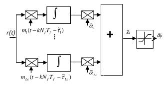
Figure 02: General structure of the Rake receiver
