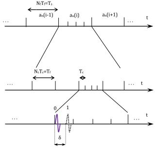
Figure 01: TH-UWB signal structure for PPM modulation
