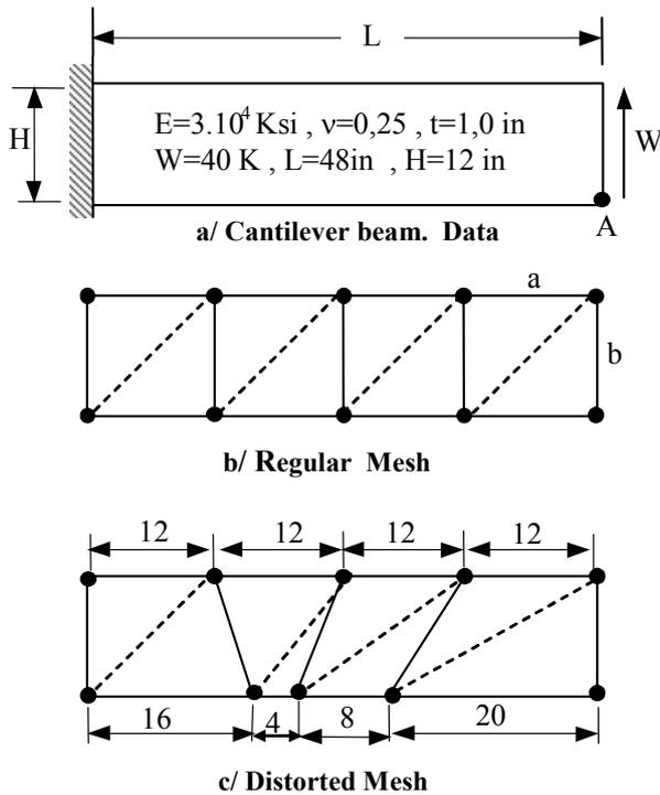
Fig.15 : Allman's cantilever beam; Data and mesh.
