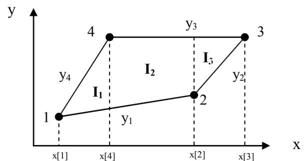
Fig 2 : Quadrilateral element
