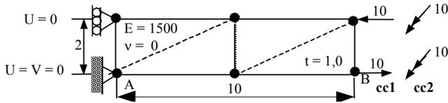
Fig. 13 : Pure bending of a cantilever beam. Data (cc = load case)
