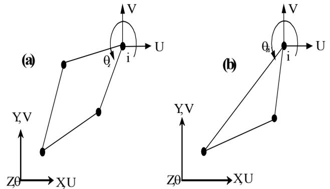
Fig 1 : Quadrilateral and triangular elements
