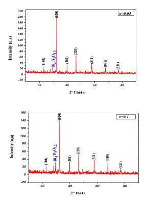
Figure 02: X-ray diffraction pattern of NBTZSN calcined at 1200 C°
