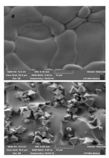
Figure 03: SEM micrograph of NBTZSN powders with the (Sb, Ni) content of (a) 5 mol% (b) 10 mol% calcined at 1200 C°
