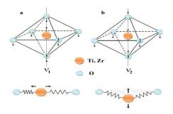
Figure 05: Schematic infrared active normal vibrations of a  $TiO_6$ octahedron, (a) higher frequency stretching vibration and (b) lower frequency bending vibration
