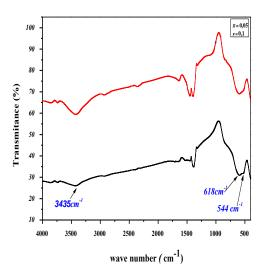
Figure 04: FTIR spectra of NBTZSN Powders calcined at 1200 C°
