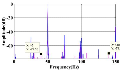
Fig.12. Second test of stator current spectrum of healthy (blue) and faulty (purple) motor at no load by FFT technique with outer raceway defect (s=0).
