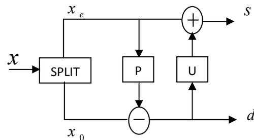
Fig. 1. Principle of lifting scheme.
