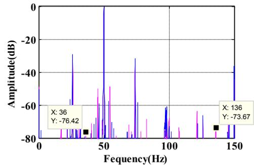
**Fig.16.** Second test of stator current spectrum of healthy (blue) and faulty (purple) motor at full load by FFT technique with outer raceway defect (s=0.044).
