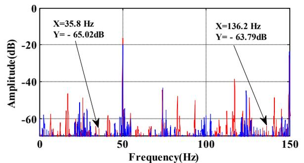
Fig.13. First test of d2 of stator current spectrum of healthy and faulty motor at full load by the lifting method with outer raceway defect (s=0.044).
