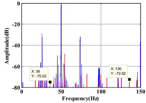
**Fig.15.** first test of stator current spectrum of healthy (blue) and faulty (red) motor at full load by FFT technique with outer raceway defect (s=0.044).
