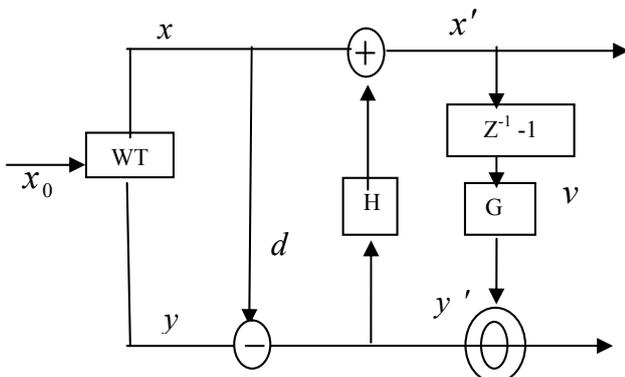
Fig. 4. Three-stage lifting scheme
