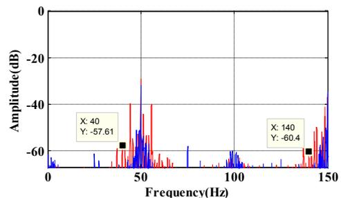
Fig.9 . First test of d2 of stator current spectrum of healthy and faulty motor at no load by the lifting method with outer raceway defect (s=0).
