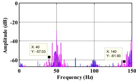
Fig.10 . Second test of d2 of stator current spectrum of healthy and faulty motor at no load by the lifting with outer raceway defect (s=0).
