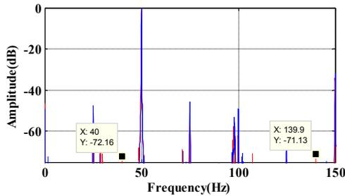
Fig.11 . First test of stator current spectrum of healthy (blue) and faulty (red) motor at no load by FFT technique with outer raceway defect (s=0).
