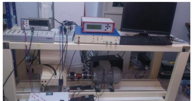
Fig.5. Experimental setup for outer race defect
