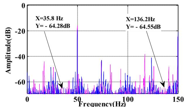
Fig.14. Second test of d2 of stator current spectrum of healthy and faulty motor at full load by the lifting method with outer raceway defect (s=0.044).
