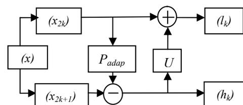
Fig. 2. Principle of lifting scheme, with non-linear prediction step before the update step.
