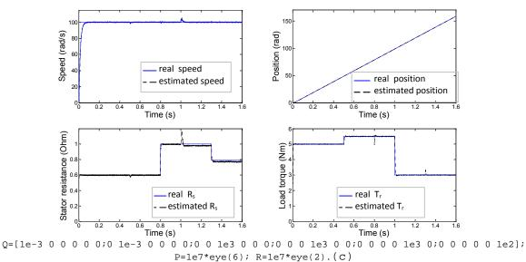
Fig. 7. Simulation results with various Q covariance matrix of system noise
