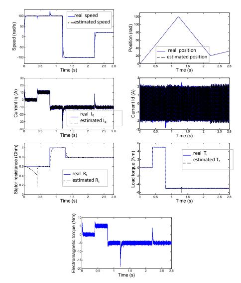
Fig. 9. PMSM estimated and actual speed, position, currents (d, q), stator resistance and the load torque with measured noisy.
