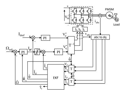
Fig. 3. Structure of control strategy of the PMSM sensorless control (Benchabane and Titaouine 2011).
