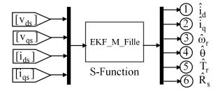
Fig. 5. Simulink based extended Kalman filter speed estimator.
