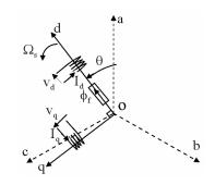
Fig. 1. Model of PMSM in d-q axis.
