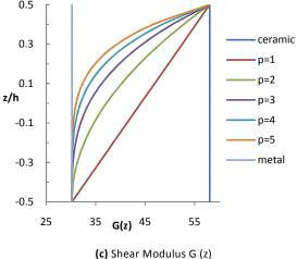
Fig. 4. Variations of Young's modulus, Poisson's ratio and Shear modulus of an FGM beam along the thickness for various power law indexes.
