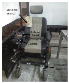
Fig. 9 . Hardware set up for the Intelligent Wheelchair
