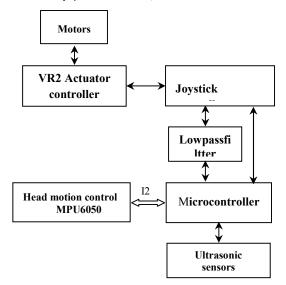
Fig. 1. Bloc diagram of the wheelchair control system.
