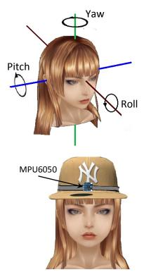
Fig. 7. Head angles and MPU6050 position
