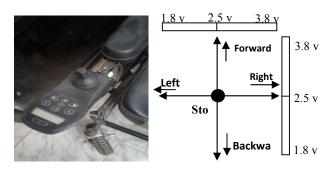
Fig. 3. The Joystick and the generated voltage from joystick axis.
