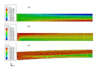
Fig 6. Nonlinear stresses states in the half concrete beam with:(a) 0 MPa, (b) 161 MPa and (c) 1286 MPa.
