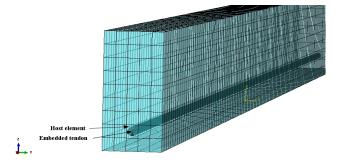
Fig 3. Finite element details of the embedded profile inside the host element.
