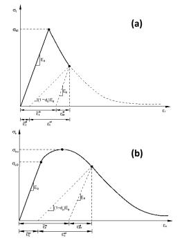
Fig 1. Stress-strain relation of the damaged plasticity model in: (a) tension and (b) compression (Abaqus analysis user's guide (2014)).
