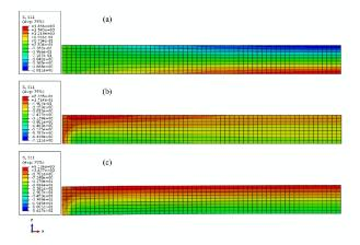
Fig 5. Linear stresses states in the half concrete beam with: (a) 0 MPa, (b) 161 MPa and (c) 1286 MPa.
