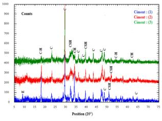
Figure 8: X-ray diffraction of cement pastes 1, 2 and 3
