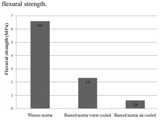
Figure6a : Flexural strength
