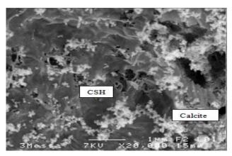
Figure 10: SEM observation of burned cement
