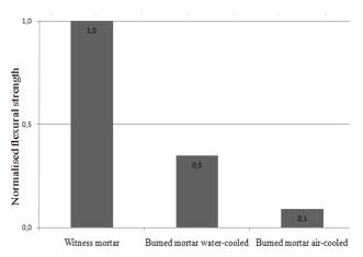
Figure 6b: Flexural strength: values normalized to the strength of witness mortar
