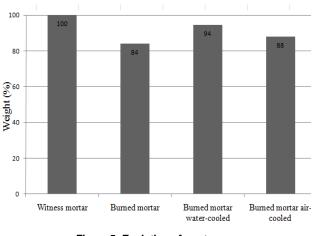
Figure 5: Evolution of mortar mass
