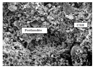
Figure 11: SEM observation of burned cement soaked in water
