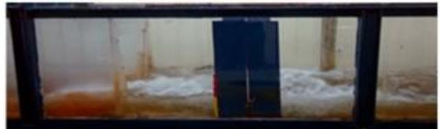
$Fr_1 = 7,07 \quad s = 10 \text{ cm}, \quad h_2 = 15,1 \text{ cm}, \quad \gamma = 1,32$
