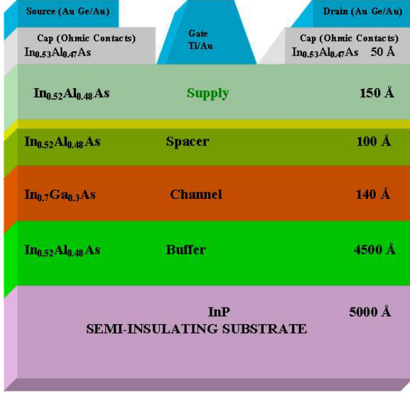
Figure 3 : The structure of the epitaxial layers of the pHEMT on an InP substrate. In the second device the semi insulating devices is made of GaAs.
