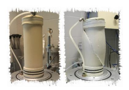
Fine particles production in sand under triaxial compression
