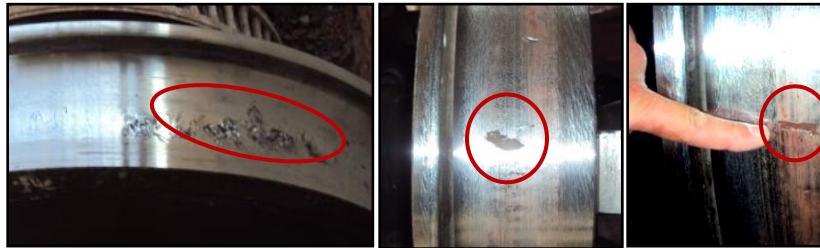
Figure1. The different defects on tread (Photos taken in the railway maintenance workshop (RMW) SMK Constantine).
